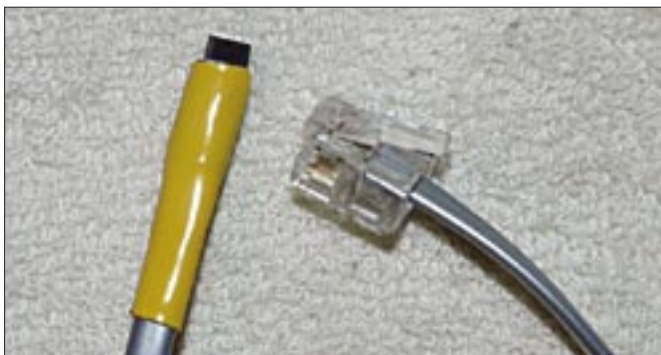
Figure 5: The finished sensor in the heat-shrunk tubing.
