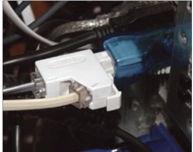
Figure 3: Two sensors connected to a one-wire USB dongle via a phone line splitter; the dongle plugs into the Linux system.
