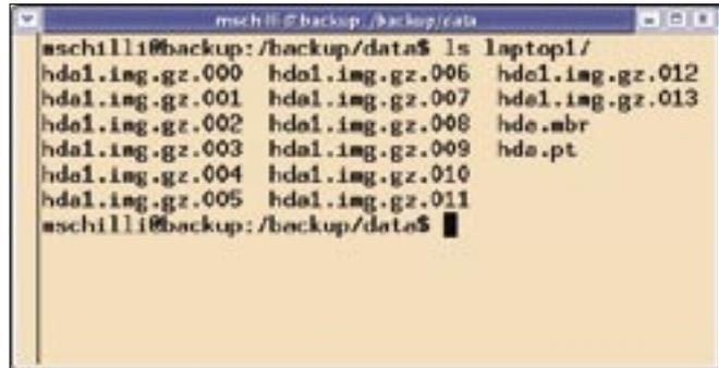
Figure 5: Backup data from a laptop with a single hard disk.
