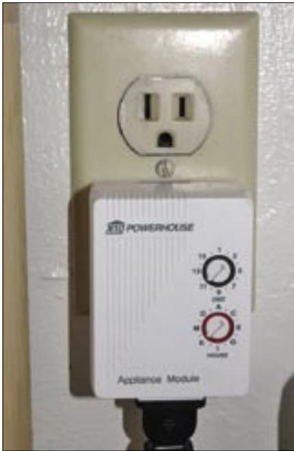
Figure 3: The X10 receiver, with the aquarium pump's power cable plugged in.
