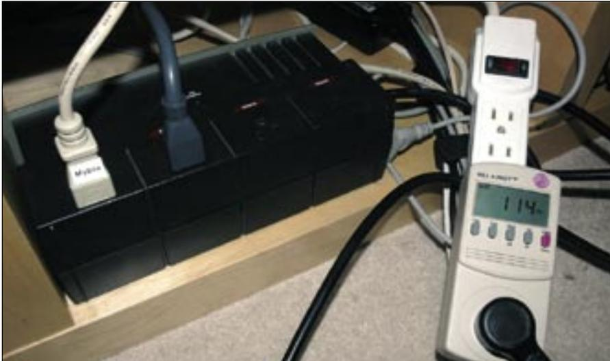
**Figure 1:** The UPS system with two power plugs on top and one serial cable plugged in on the right. The “Kill-A-Watt” meter indicates that PC, DSL modem, and router combined are using about 114 watts.
