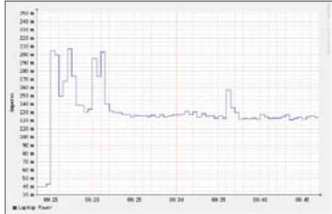
Figure 4: Power consumption of a laptop shortly before and after switching on.
