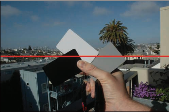
Figure 1: Discovering the color values for the three cards in the picture - the script reads the RGB values along the horizontal line at the center to obtain the graph in Figure 2.
