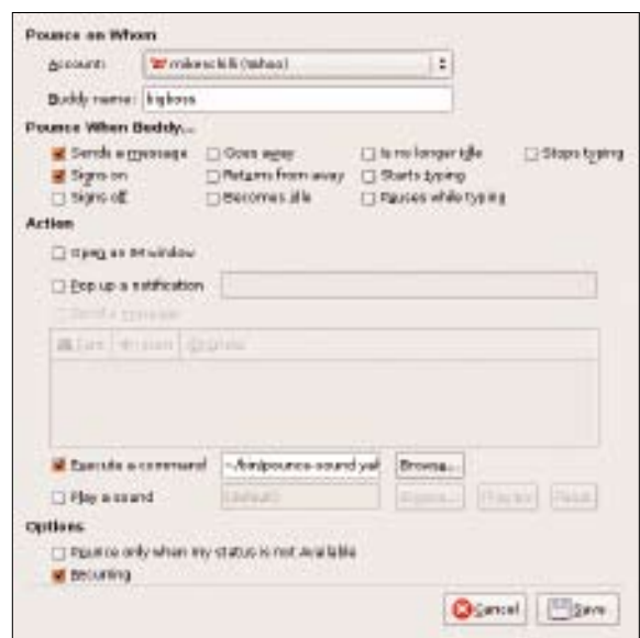
Figure 1: The “Pounce” function in Pidgin runs the ~/bin/pounce-sound script when IM buddy “bigboss” triggers an event.
