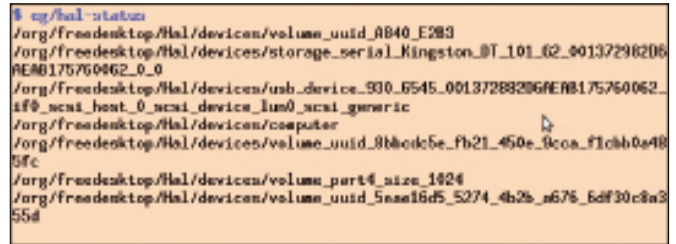
Figure 2: Net::DBus connects with the system D-Bus and outputs all hardware components detected by the HAL Manager.
