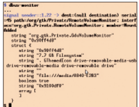
Figure 3: News of a recently plugged in and mounted USB stick is propagated on the D-Bus.
