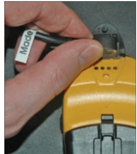
Figure 2: A special connector lets you hitch up the eTrex to your PC’s serial port.
