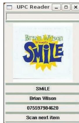
Figure 4: The scanner identifies CDs and DVDs by interpreting the UPC code and retrieves the product data and cover image from Amazon.com.
