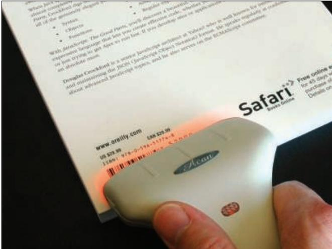
Figure 1: The barcode scanner can read the UPC or EAN code on a book.
