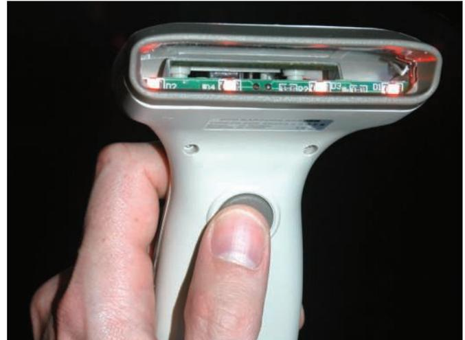
Figure 2: The scanner has a CCD sensor and switches its red diodes on at the push of a button.
