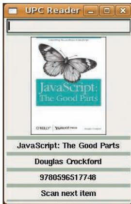
Figure 3: The script has sent the scanned code to Amazon.com and received the product data in return.
