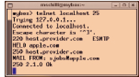
Figure 4: ... and the client can then exchange SMTP commands as if connected directly. The server thinks it is talking to a local client.
