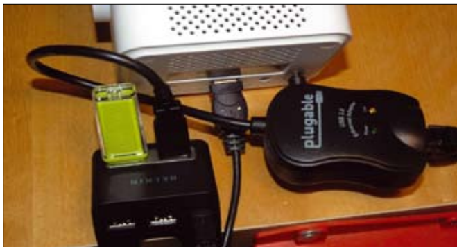
Figure 3: The USB hub connects my Chumby with an Ethernet adapter and holds the memory stick with the user hook file that contains the proxy settings (Figure 4).
