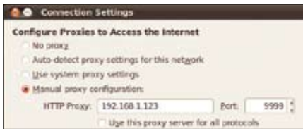
Figure 6: The Firefox Connection Settings dialog points the browser at the modifying proxy.
