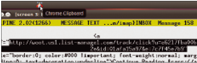
Figure 1: The Perl script hiding behind the propeller hat grabs the URL from the primary text selection and launches Chrome with it.
